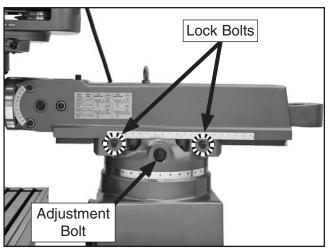
**Figure 24.** Ram forward/backward movement controls.
